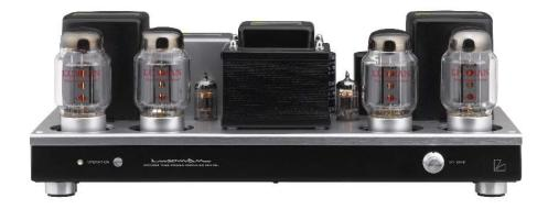
The MQ-88uSE is based upon the legendary and much sought-after MQ-60 stereo power amplifier. It utilises KT-88 valves from Slovakia JJ Electronics, configured in triode mode. Extensive research has delivered perfect circuit stability, integrating miniature JJ-made valves into the amplifier and oil condenser connections. This has resulted in an even smoother tonal quality, coupled to powerful scale and drive.
