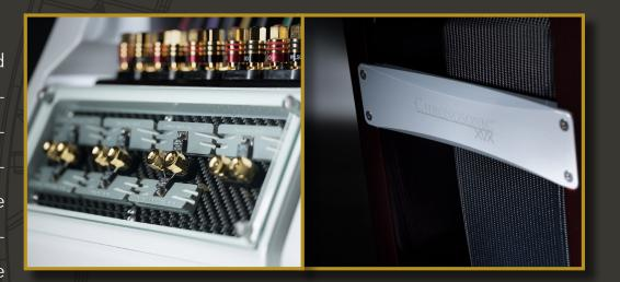
XVX. The tuning and protection resistors are located on an easily accessible portion of the rear cabinet. Each is mounted to a carbon fiber substrate. Changing resistors is a simple matter of removing a quick-release glass cover and removing the hardware from the heatsinks.
