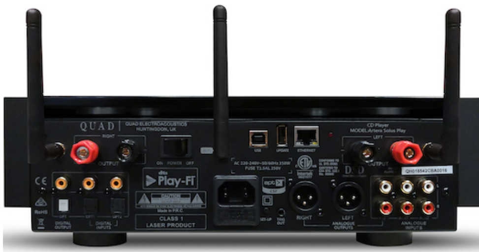
Flexible friend Around the back, three aerials – two for Wi-Fi, one for Bluetooth – and a plethora of inputs and outputs highlight the Artera Solus Play's versatility
