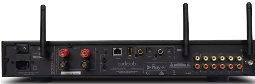
Around the back are three aerials for Wi-Fi and Bluetooth, plus a wide range of analogue and digital cable connections
