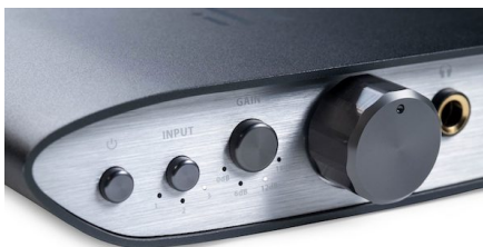
To the left of the aluminium volume control are three buttons: power on/off, input selection and gain selection
