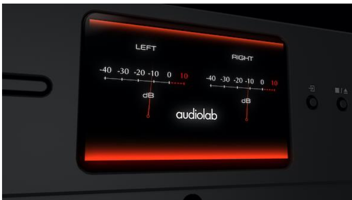
Left The Omnia's 4.3in screen can display an analogue-style VU meter
