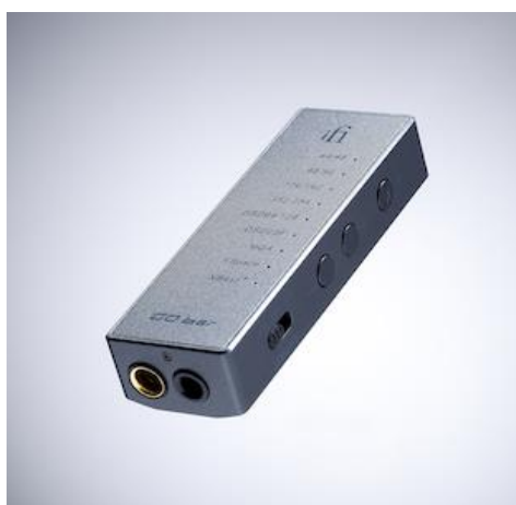
Left The GO bar's robust yet lightweight alloy enclosure sports a range of useful LED indicators, controls and even a balanced output
