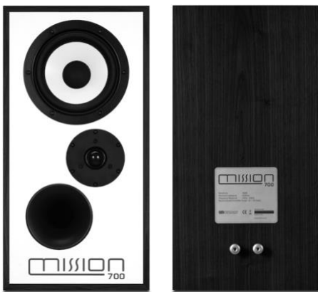
Left New Mission 700, front and back. Note the IDG arrangement, with the tweeter offset below the mid/bass driver, and the front-firing port sited beneath
