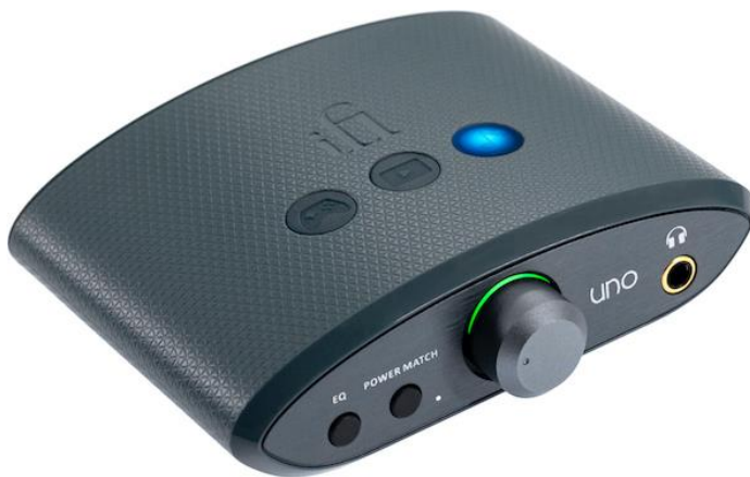
Left Three illuminated logos on the Uno's top surface indicate which analogue EQ mode is engaged: Music, Movie or Game
