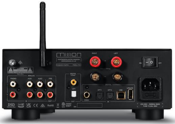
Left The 778X's rear panel packs in an impressive array of digital and analogue inputs and outlets
