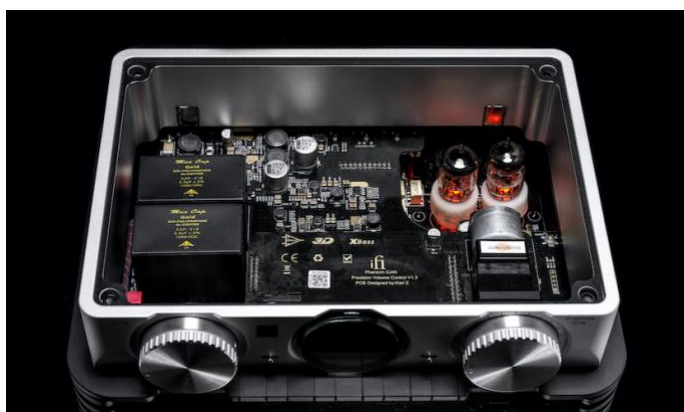
Left The iCAN Phantom's meticulous, multi-level circuit board layout features True Differential Balanced design
