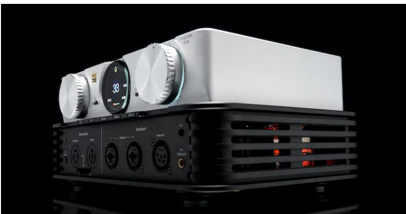
Left The iCAN Phantom's black lower section offers a plethora of connection options front and back
