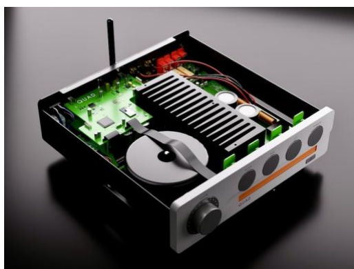
Left QUAD has utilised every inch of the amp's chassis to pack in top-quality circuitry without compromising the internal layout
