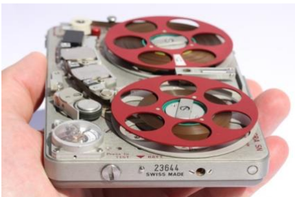
Left Originally a top-secret CIA commission, Nagra's SN is the archetypal sound recording device for Cold War surveillance
